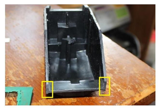
Line up the hopper and the tank. Make sure there's enough gap between the tank & the hopper for the back, I used a piece of the stock I intend to use to make the back to measure. If the space is too small, file the back of the hopper till there is.
