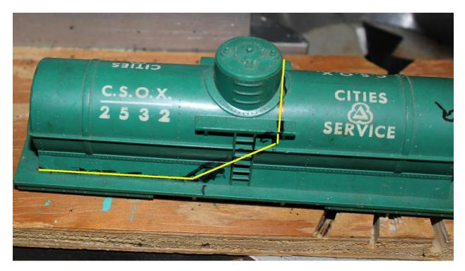
I use a larger diameter wheel and cut from the back side of the dome. Make this cut as close to the dome as you can and as straight across as possible.
