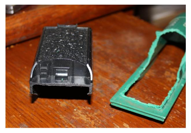
Don't sand either of these ridges off, the cat walk sits on top of them. The next step is to remove the molded ladder from each side by first scraping it with an Xacto knife, then sanding it smooth. I'll work on that tomorrow
