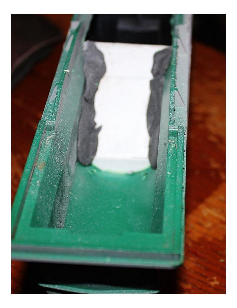
The steel stik sets up quickly so smooth it out quickly and it won't need sanding. Fill in any small gaps with squadron putty or whatever your favorite filler is. Sand it gently. Try not to sand away any of the molded detail if you can
