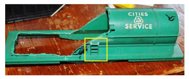
After getting the ladder sanded, glue the hopper to the tank car frame. Super glue works best as it's thinner but line it up quickly! JB Weld "Gel" superglue gives you a little more time.
