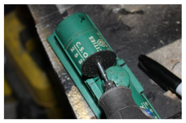
I use a thinner cutting wheel to cut the angle on the sides and around the frame, Be careful as the frame can be broken quite easily at this stage.
