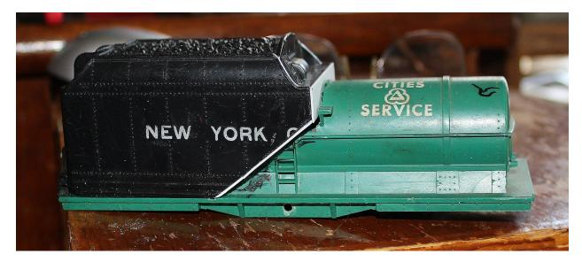
I decided to keep the undamaged part of the ladder, you can also remove it if you want to. A dremel with the small sanding bit will remove the bulky parts, then trim and peel any extra away with a xacto knife, sand smooth. It's easier to fix or remove the ladder before gluing the hopper.
