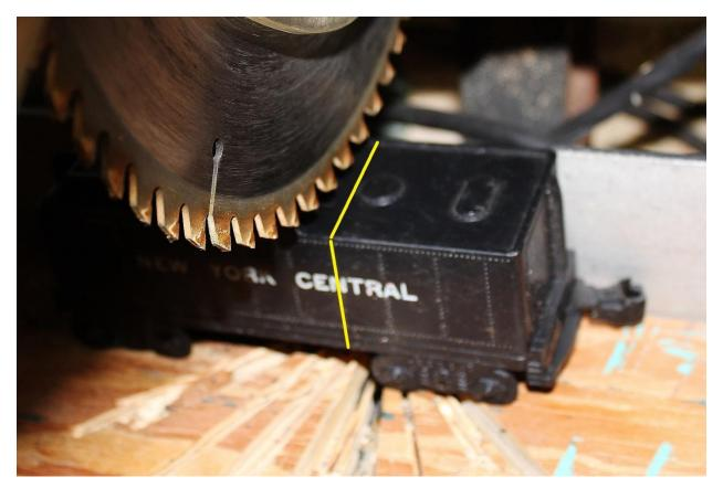
After the tender is cut, then cut the faux molded wheels from each side with a dremel and thin cutting wheel. Cut about on the red line. Leave a little "wiggle" room as the cutting wheel tends to melt the plastic a little as it cuts. Then sand the cut smooth with the bottom of the tender with a round sanding wheel. Use the chop saw to cut the angle cut. Draw a line with your permanent marker from just above the lettering to the rivet line (the one that goes through the "R" as shown.
