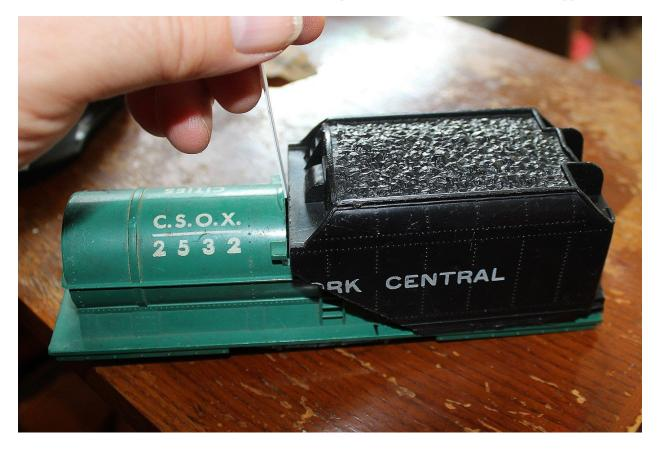
Line up the styrene strip to make the shorter piece first. I used plastruct styrene strips #90642 (.030x 1 1/4") for mine. After marking both sides, cut with a straight edge & utility knife or a guillotine type cutting board. I have one I bought for scrap booking that works great.
