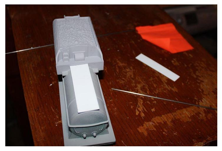
I drill my railing holes first, then bend the wire to fit, I don't know what size bit I use, I eyeball it by lining the base of the bit up with the wire.
