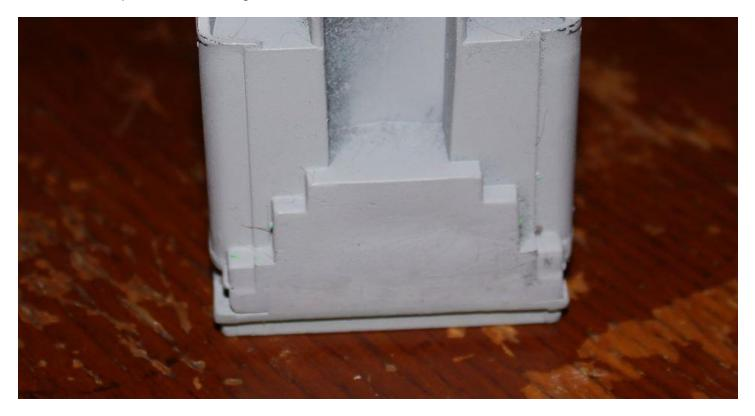
Lightly sand away the lettering, being careful not to sand off the molded rivets. Then cover with the Rustoleum primer and it will smooth out any sanding marks or scratches.
